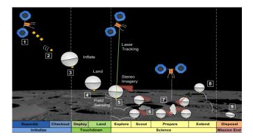
The complete AMIGO concept relies on a mother spacecraft deploying (1) multiple AMIGO landers that descend towards the asteroid's surface. Before touchdown, each AMIGO inflates a 1 m sphere (3). On the surface, a stereo camera on top of the sphere collects observations (5). After sufficient observations are collected, each AMIGO can hop to a new area (8) via microthrusters and a reaction wheel. Credit: Wilburn et al. 2019, Figure 4.
